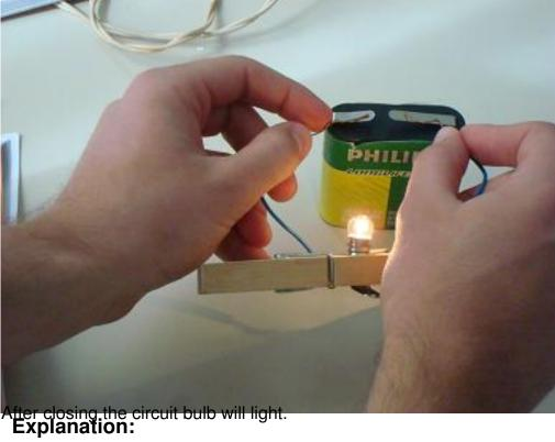
Electrical current flows from the guides of higher potential to lower potential. To make this possible, in a closed loop must be an element that ensures supply of charge carriers of the points with a lower
